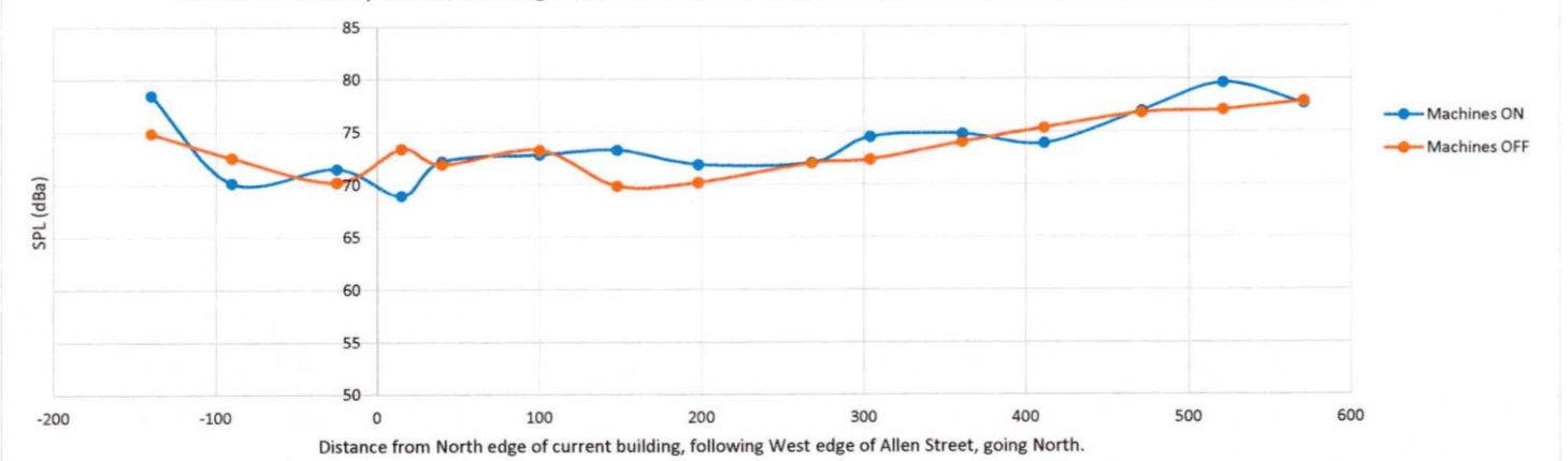
Sound level comparison, readings from EXTECH 407730, wind screen on, max hold, 30 second observation.
